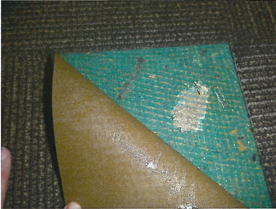
9. Non-ACM green mastic beneath 2' x 2' carpet squares (CM2-Samples 21, 22, 102, 103) in Office 164.01.
